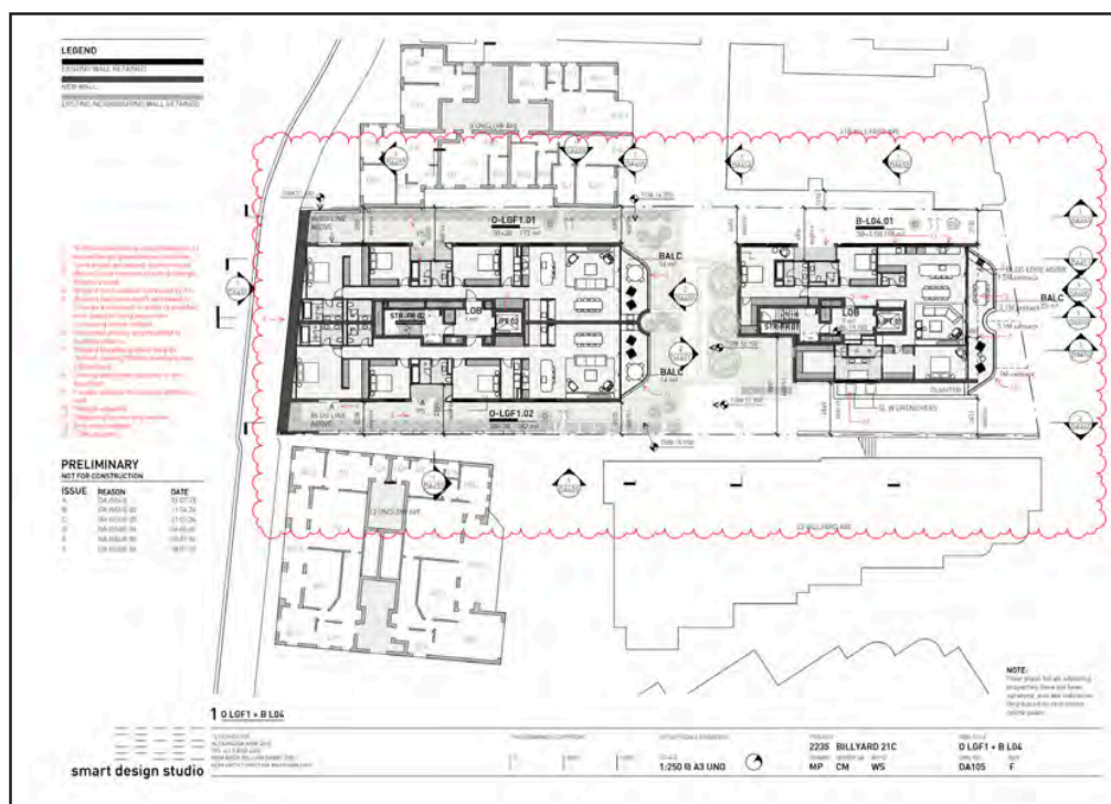
Figure 4 – Typical floor plan of proposed design by Smart Design Studio - extent of revisions indicated within red cloud.
